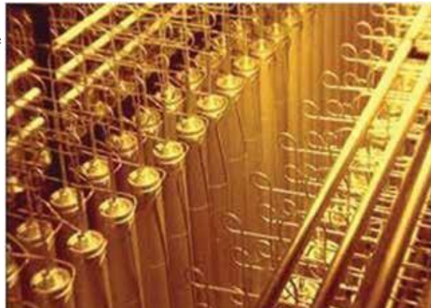
Gas centrifuges can be used to enrich uranium and are subject to nuclear nonproliferation (NP) controls
